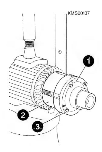
Assembling intermediate bearing
